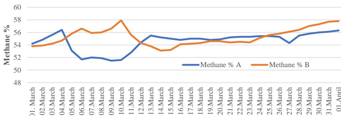
Fig. 2. Methane contents % in biogas from bioreactors A and B
