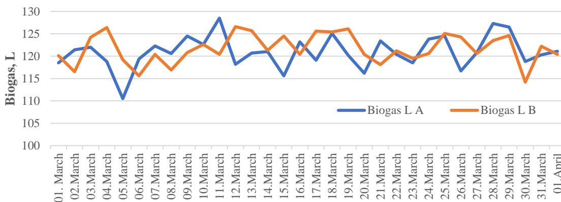
Fig. 1. Biogas production in bioreactors A and B
